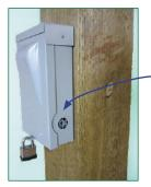
Appendix 1 in the counter's instruction document explains how to house the counter in a low-cost (\$15), lockable electrical box. Download at: www.trafx.net/support
