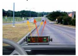
The direction sensing ability of the Stalker 2X allows the operator to select a specific direction of traffic to monitor. The 2X can measure closing targets while automatically ignoring vehicles that are going away-even if the target moving away is closer than a distant closing target.
