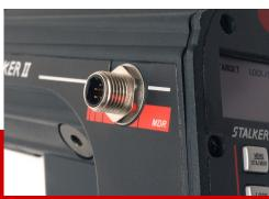
The Stalker II MDR can be purchased with an optional rear antenna port. With this feature, a second, rear-facing antenna can be connected to the Stalker II MDR to yield the performance of a two-antenna dash-mounted unit either in a patrol vehicle or on a motorcycle.
