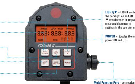
**LIGHT**/▼ - **LIGHT** switches the backlight on and off. ▼ sets distance in stopwatch mode and decrements settings in the operator menu.
